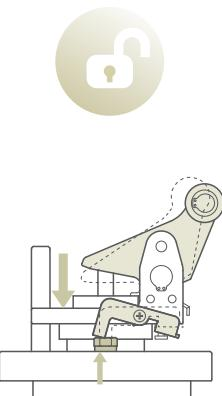
Pneumatic unlock lock mechanism
