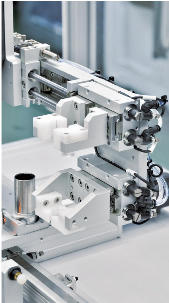
Parallel gripper MCHD ▲ / MCHU ▼ for automatic assembly of gripping applications.
