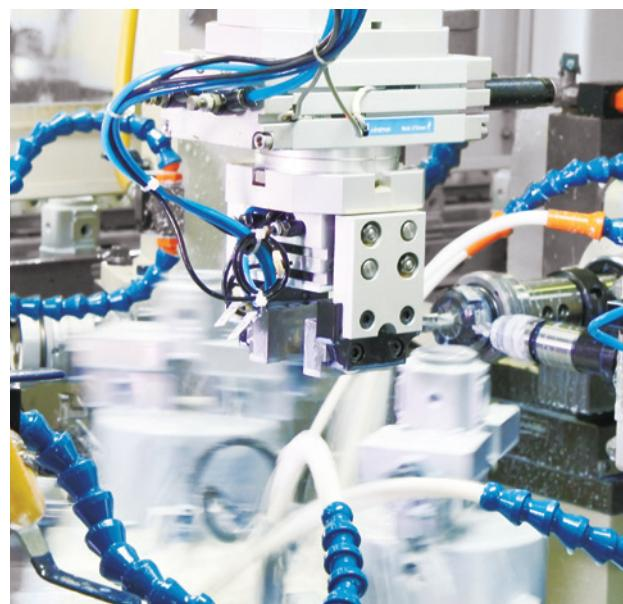
Rotary actuator MCRQ with gripper MCHX for machine tool application.
