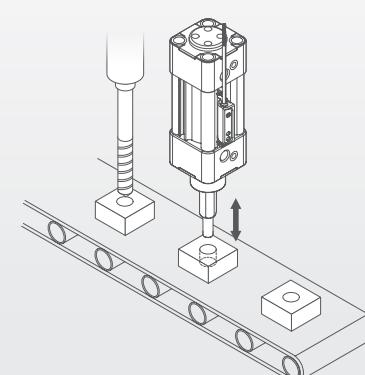
Used to check machined holes.
