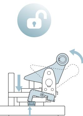
Pneumatic unlock deactivation mechanism
