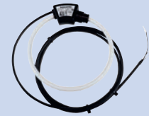
ROG 131 mV @1 kA, 2 wires Up to 4000A
